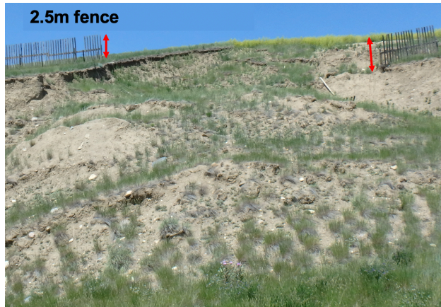
Figure 13 View of the upper half of the Chin Coulee landslide showing a 2.5m high fence as reference scale for the dimensions of the back scarp
