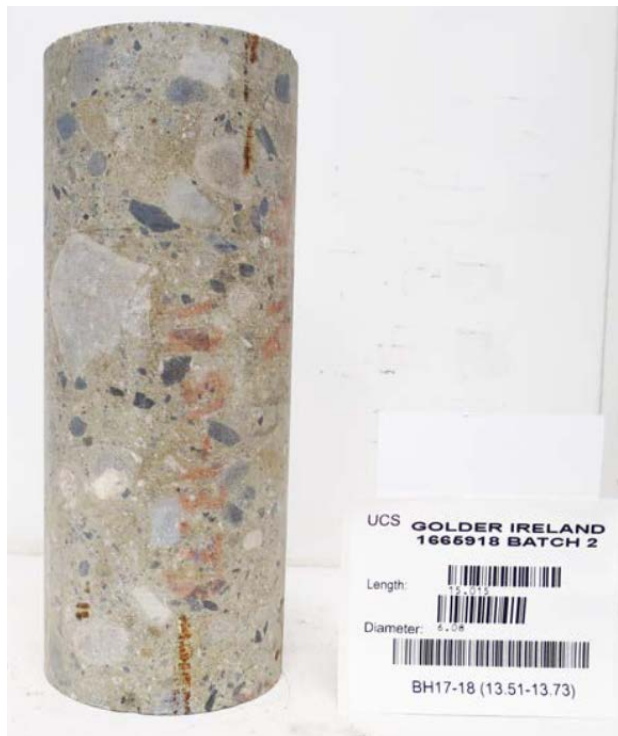
Figure 4. A sample of volcanic Breccia rock core before being tested. Core extracted from borehole next to pier 18.
