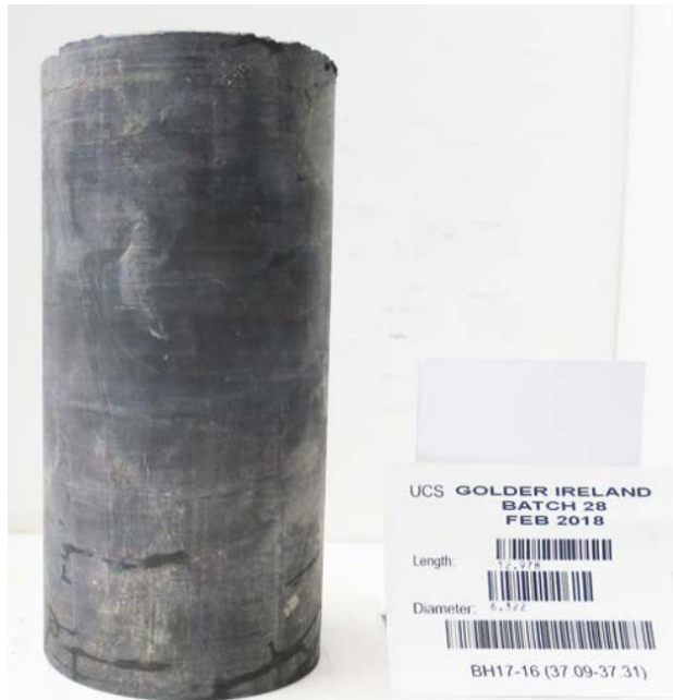
Figure 3. A sample of Shale rock core before being tested. Core extracted from borehole next to pier 16.
