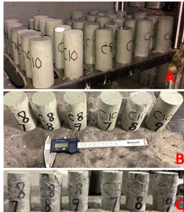
Figure 3. A) Samples while in the moisture room, B) and C) one set of samples before testing and after, respectively.
