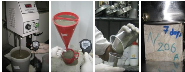
Figure 4. Some measuring sets for two-component grout test (Novin et al. 2015)
