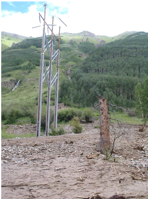
Figure 2. Deposit from a 2011 debris flow near Ophir, Colorado, USA. A snow avalanche also reached the site, but the deposit has melted. Photo: C. Wilbur.
