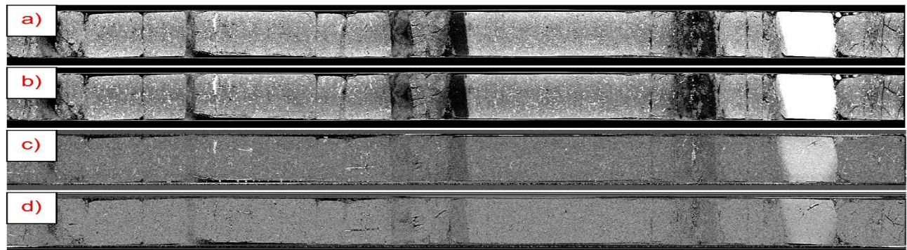
Figure 5. Example of Dual Energy scan images from Mile 184.4 Site: (a) low energy whole core scan, (b) high energy whole core scan, (c) reconstruction based on atomic number, and (d) reconstruction based on bulk density.
