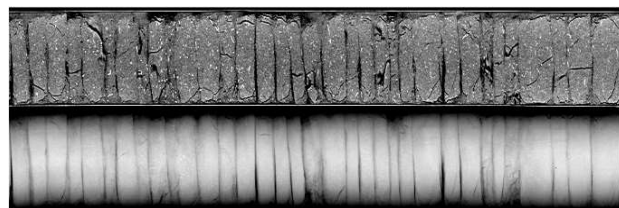
Figure 7. Example of mechanically damaged core.
