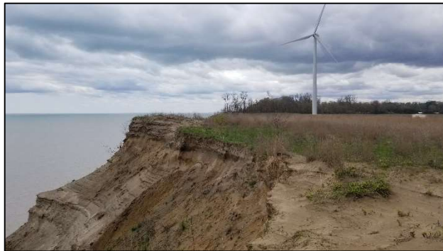
Figure 7. The shape of the bluff face can be seen in this side view photo taken during the initial site visit. Another turbine can be seen in the background.
