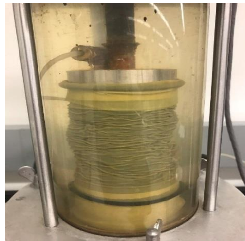
Figure 7. General bulging at \sigma'_3 = 100 kPa
