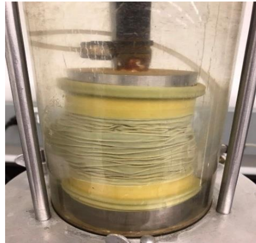
Figure 6. Lateral bulging at \sigma'_3 = 80 kPa
