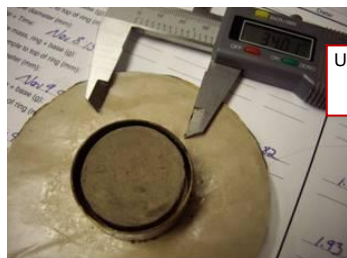
Figure 2 Use of a micrometer to measure volume at various degrees of drying.
