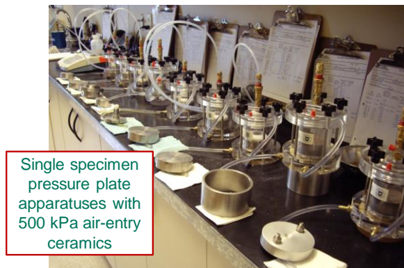
Figure 5 Series of Pressure Plate Cells measuring water content versus matric suction.
