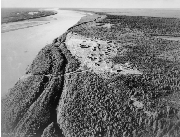
Figure 7. Looking north towards Fort McPherson in the 1930's. Note apparent removal of trees and shrubs in and below the developed part of the community, and the locations of overflow/creek channels in the floodplain. (Photo credits: Glenbow Archives NA-3844-92; or National Air Photo Library A2653-10; used with permission.)
