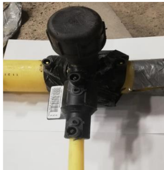
Figure 1. Tee-joint used for branch connection
