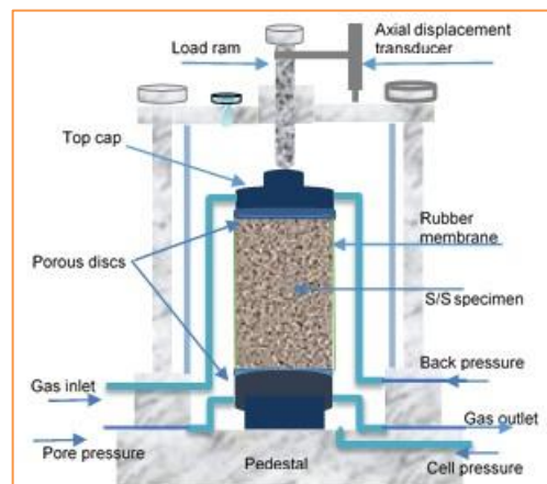
Figure 2. Cross-section of the modified triaxial cell
