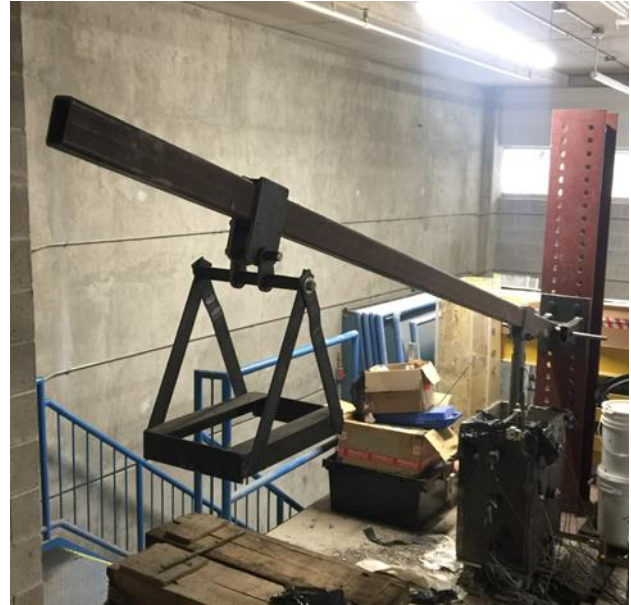
Figure 2. Experimental set-up of large-scale consolidation test.
