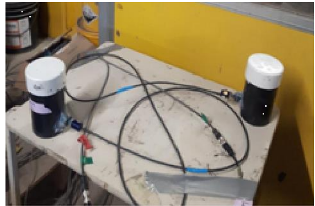
Figure 5. Two T5x tensiometers installed into two replicate columns.
