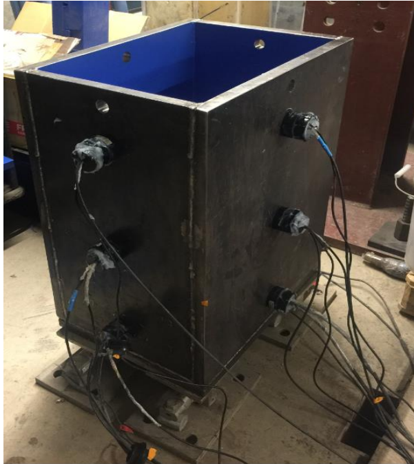
Figure 3. Steel box showing pore-water pressure and volumetric water content sensors.
