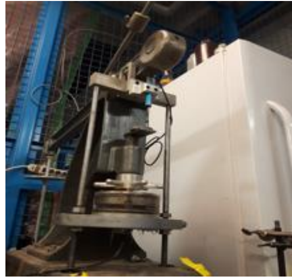
Figure 4. Modified oedometer with T5x pore-water pressure sensors installed in the base and connected to DL 2e data logger.
