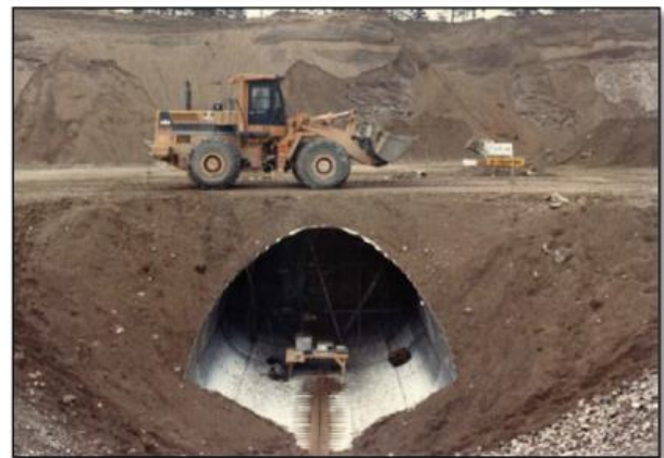
Figure 2. Full-scale pipe test in Enköping, Sweden (Pettersson, 2007)
