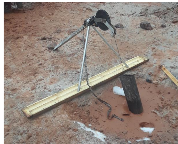
Figure 10. Televiwer surveys of the TV19-08 hole
