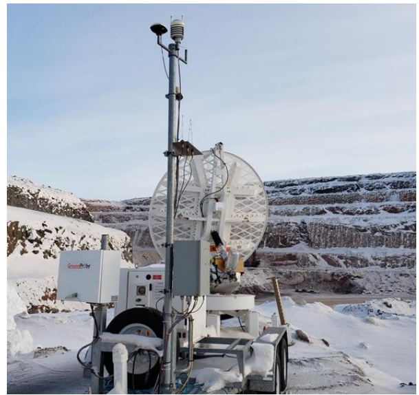
Figure 23. Slope Stability Radar monitoring the southeast wall
