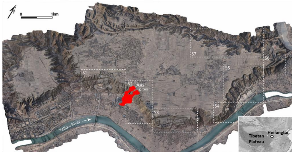
Figure 1. Landslide distribution along the margin of the Heifangtai terrace (HFT) showing 7 sections that are dominated by different types of landslide. Locations of the DC#2 and DC#3 flowslides are shown.
