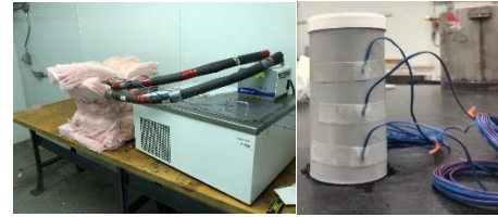
Figure 2. Temperature control system and instrumented dummy sample in a mold
