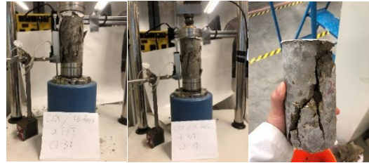
Figure 11. Failure plane in C2 soilcrete specimens: the left is a specimen cured for 56 days exposed to 2 F/T cycles failed on loading frame; the middle is a specimen failed at 56 days of curing with exposure of 4 F/T cycles; the right is a specimen failed at 110 days of curing
