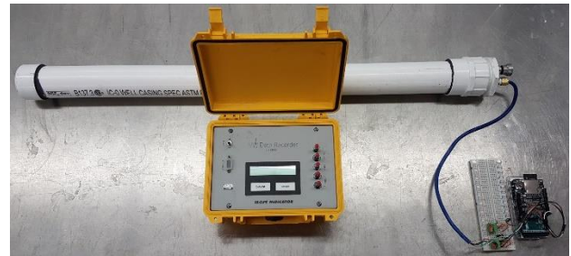
Figure 3. Pressure chamber with commercial readout unit and low-cost datalogger
