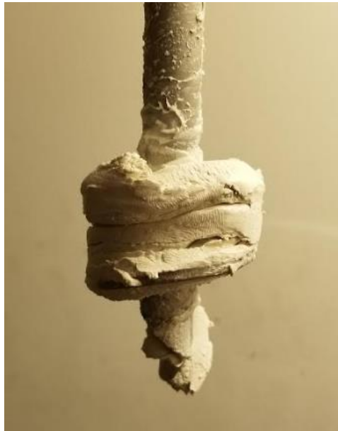
Figure 1. A model pile extracted from the clay
